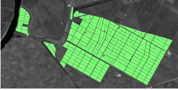
Figure 1 Illustration of agricultural fields labelled as Rice fields (in green), over a Sentinel-1 \sigma_0 temporal average image, in VV polarisation, of the BXII Sector (36°59 N 6°06W)
